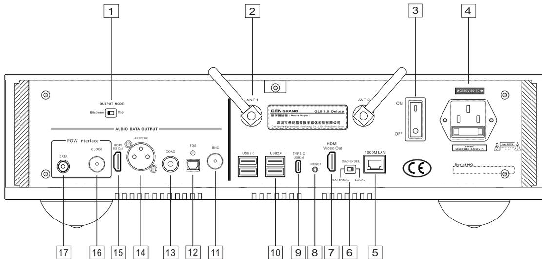
1. **Output Mode Selection Switch:** If you are using the **POW** interface or I2S to output data to a DAC, the switch must be set to "Bitstream". If you are using SPDIF to output to a DAC, the switch must be set to "DOP". Otherwise, noise may occur.
